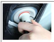
6. Inflate the **Oxygen Air Frame** until you can give it a 'good squeeze'; the tube requires room inside for air to expand, should there be any fluctuations in the ambient temperature. Don't be concerned if you do keep inflating, however, as the **Intelligent Frame Relief Valve** will release any excess air above 6PSI.
