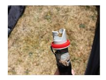
4. Next, attach the pump to the Dynamic Speed Valve and begin to carefully inflate - taking care that no part of the fabric is caught anywhere.
