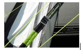
13. Finally - thread the draught skirt through the lower awning channel and secure at either side.
